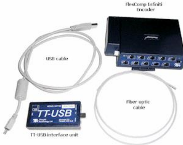
Unconnected hardware components
